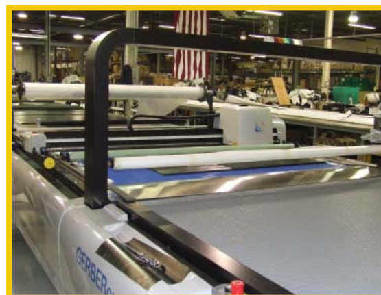
Multi-ply fabric cutter at the Orangeburg facility is capable of cutting up more than 15 layers of fabric simultaneously.
