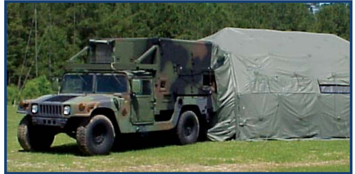
A Humvee using a T-Boot to attach to a DRASH 4XBT.
